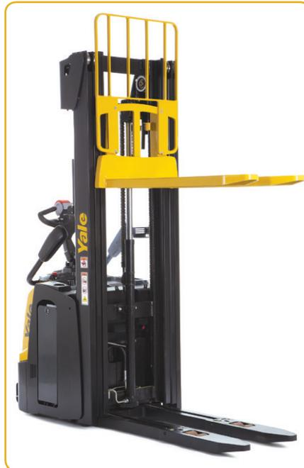
The adjustable pull rods give uniform lifting and lowering movement of the forks. The loading rollers are tandem with lubrication points and sealed bearings. Speed is automatically reduced with load arms raised.
