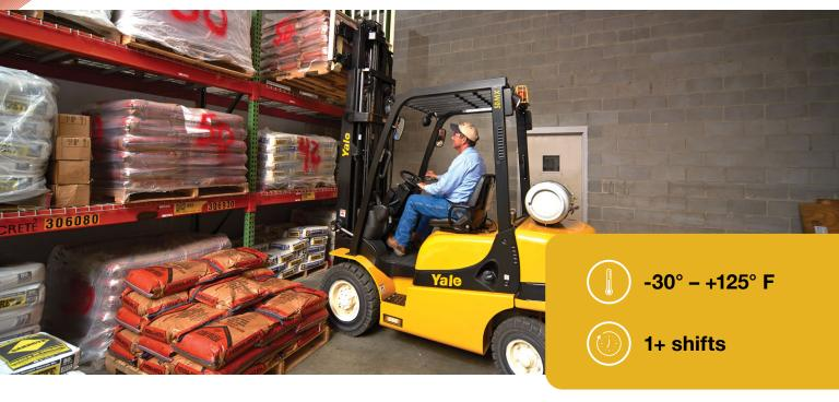
Internal combustion engines (ICE) keep lift truck power simple and easy, with fast refueling, minimal indoor space requirements for fueling infrastructure and strong power delivery until full depletion.
