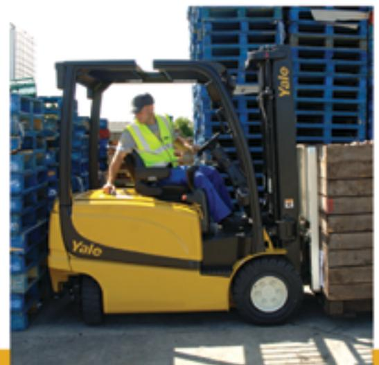
The ERP-VL series combines proven AC technology with the innovative “Extended Shift” function to provide an excellent balance between battery run time and truck productivity. This highly efficient system provides longer battery run time for increased throughput, and the “Extended Shift” can be disabled for increased productivity.
